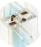
Within the head of the frame is an anti-lift block which prevents the doors from being lifted out of the frames.
