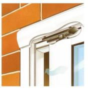
Four locking bolts locate behind keeps made of heavy grade stainless steel which prevents the door being forced away from the frames.
